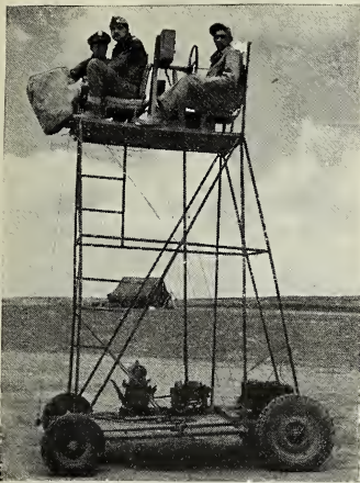
The improvised bombardier trainer (above) made from salvaged materials by a B-26 squadron in North Africa. The "inventors" of the contraption are (left to right) Lieutenant G. K. Rhodes, Captain Joseph F. Perrin and Tech. Sgt. Herbert W. Eckhardt.
